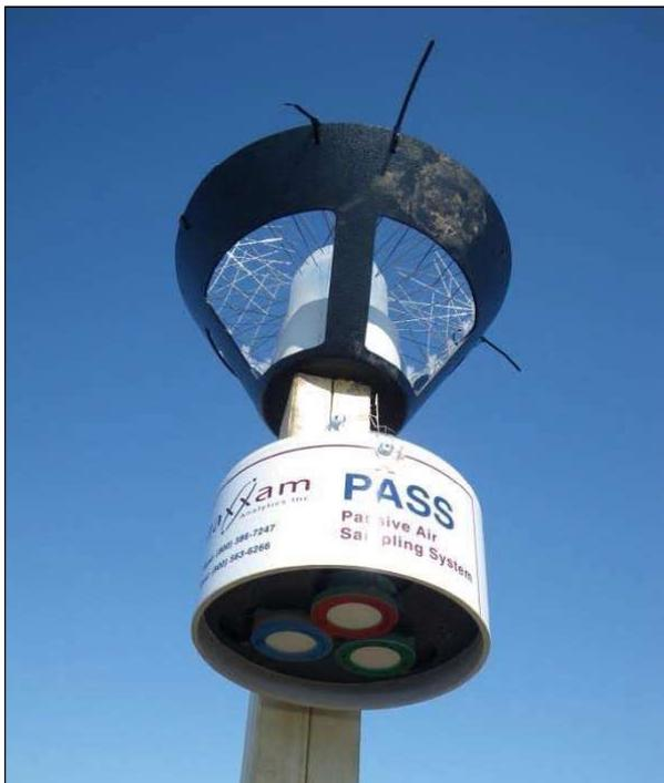
*Plate 2. Pass Filters in Rain shelter attached to wood dustfall stand.*
