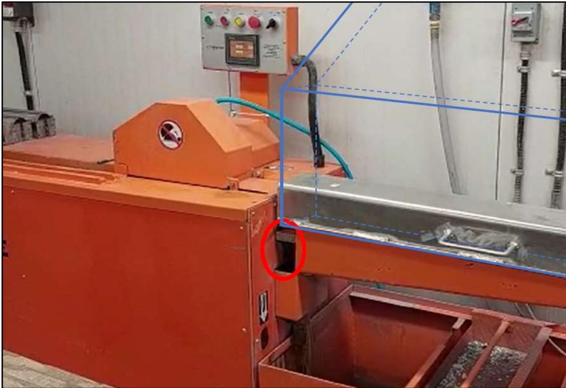
**Figure 2: Main Fugitive Dust Escaping Location (after VETS)**
