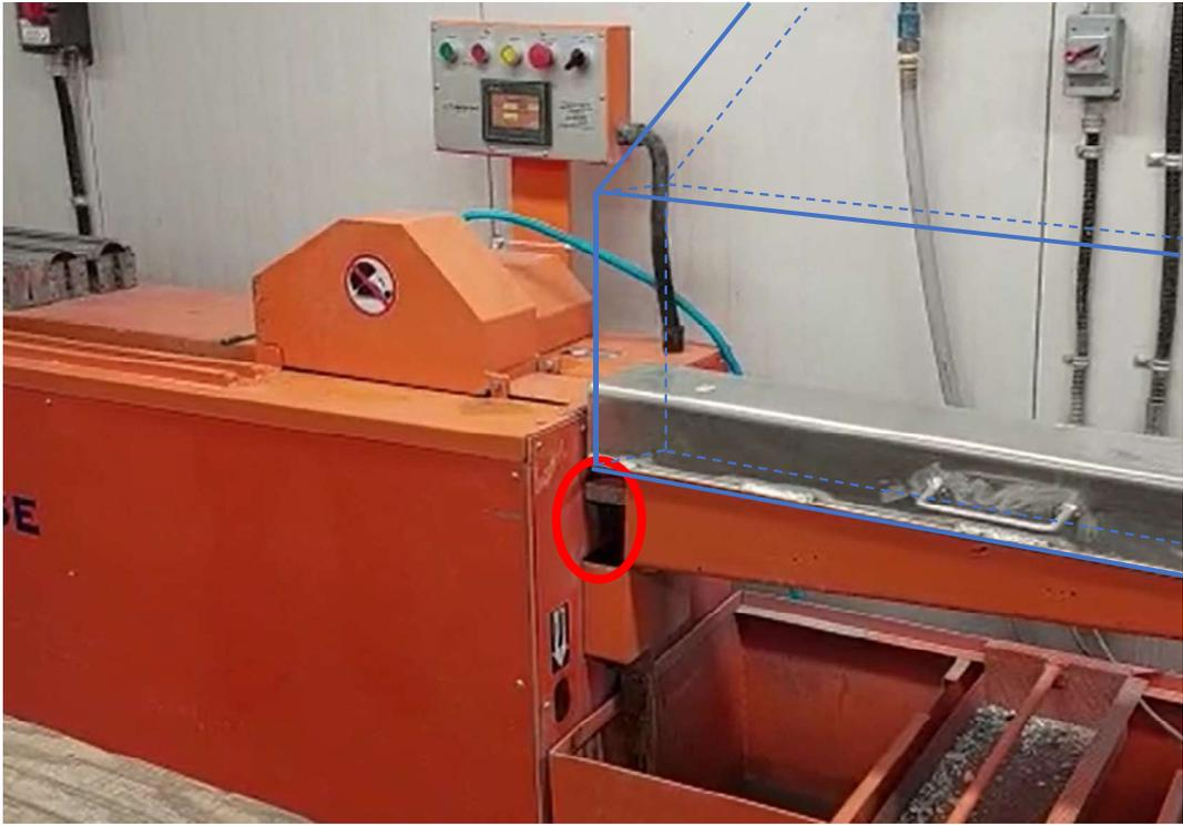
Figure 1: Core Saw – Location of Fugitive Dust
