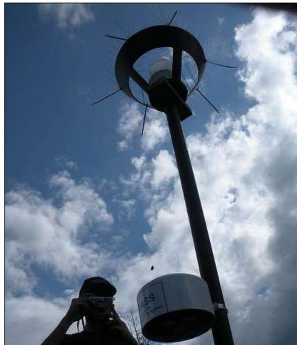
*Plate 3. Pass filters in rain shelter attached to metal dustfall stand.*
