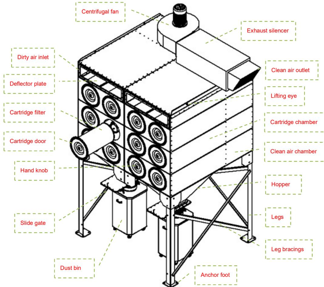
**Construction:** Material: Carbon steel, Stainless steel or Galvanized steel
