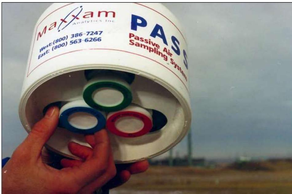
Plate 1.  $\text{SO}_2$ ,  $\text{NO}_2$ , and  $\text{O}_3$  sample filters attached to the rain shelter.
